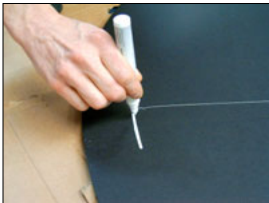
Figure 7. Drawing a circle to mark the inside of the perimeter band.
