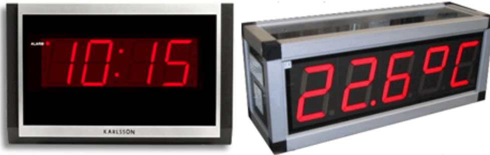
Figure 5. Devices that have seven-segment displays.
