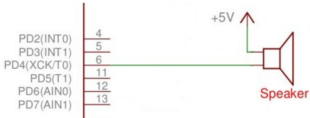
Figure 3. Piezo speaker circuit schematic.
