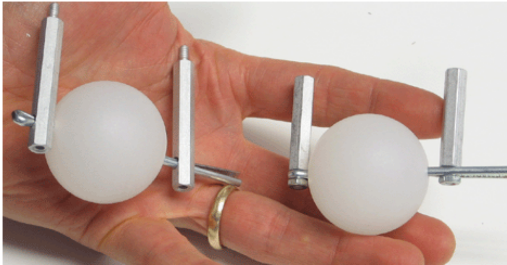
Figure 5. Two ways to mount the cotter pin and plastic ball.
