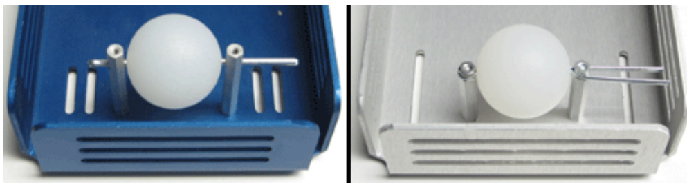
Figure 6. Caster secured to robot chassis.
